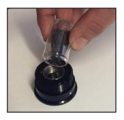
3. Pour powder charge into stainless High Pressure Chamber
