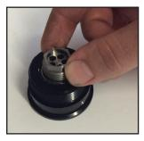
5. Install stainless vent plug and snug up with 15mm wrench
