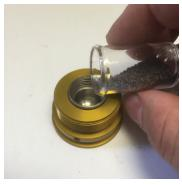
3. Pour powder charge into stainless High Pressure Chamber
