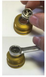
5. Install stainless vent plug and snug up with 15mm wrench
