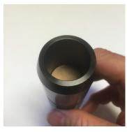
7. Install cardboard or foam disk to secure payload pushing wad into bottom of tube
