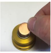
4. Install copper burst disk (sharp edge up) covering powder charge and resting on High Pressure Chamber ledge
